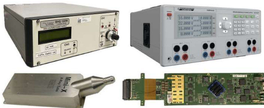
Figure 5: Experimental setup components (The high voltage supply (top left); the power supply for the board (top right); the X-ray tube (bottom left); the high voltage board (bottom right))
